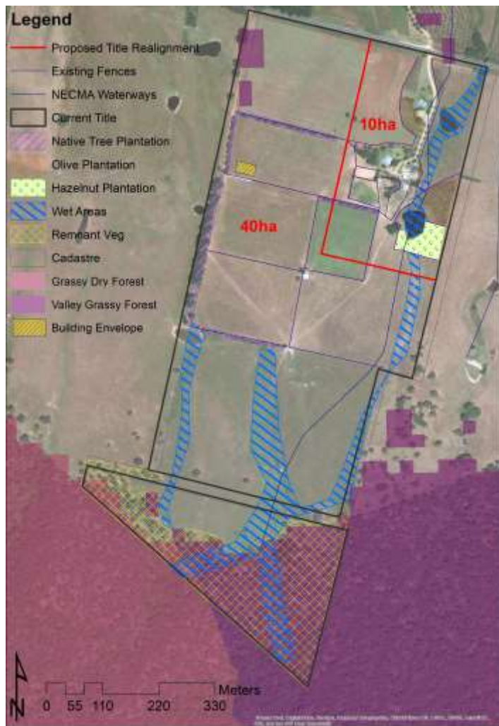
Figure 1: Shows the subdivision layout on site.
