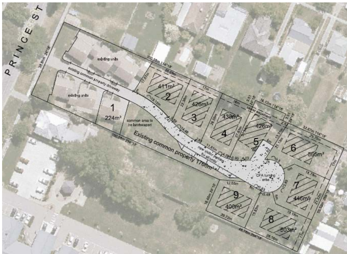
Figure 3: Shows the development layout on site.
