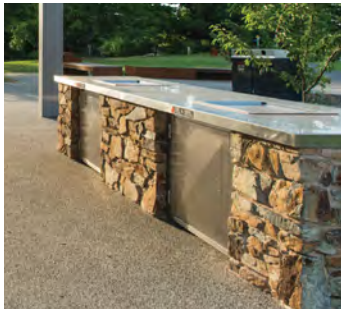
[BQ] Electrical BBQ Supplier: Christie Parksafe, Modular Triple Product Code: HMOD-E-3.2 Material: Brushed stainless steel finish with local stone cladding Features: 3 Module Installation Kit with 2035mm x 750mm Stainless Steel Bench, 2 x Electric Stainless Steel CCQ cooktops, Safety Push Button Start Timing Control. Installation and connections in accordance with manufacturers specifications
