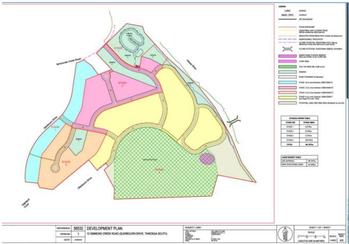
Figure 5: Shows the development layout on site including the road network, pathways along the eastern edge and stages of development in yellow, orange and pink with reserves/no build areas in green.
